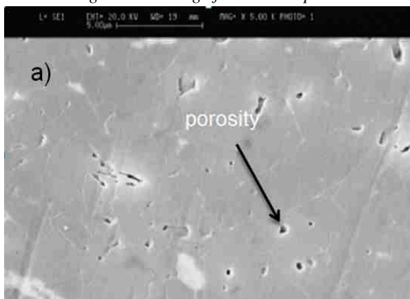
Fig.5. SEM Image for sintered composite %94 Al-%2 SiC-%4 ZrO 2
